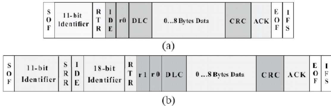
Figure 3.2: (a) standard CAN frame, (b) extended CAN frame, taken from [34]
