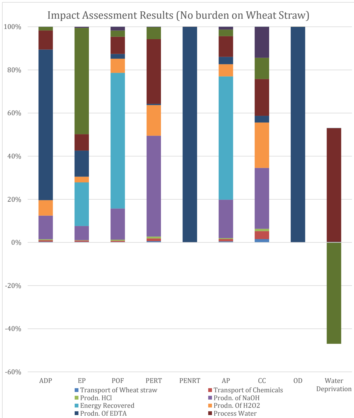
Figure 4.3: Contribution of different processes to the different impacts with no burden associated with wheat straw
