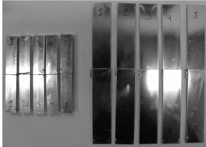
Figure 31 - Joined test specimen, 5 rods to the left, 5 metal sheets to the right.
