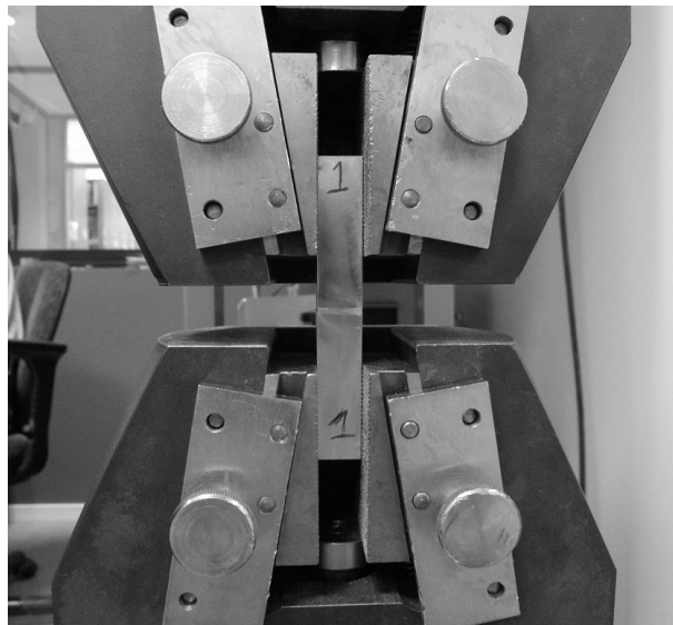
Figure 32 - Fixture of tensile test rig with tensile sample.
