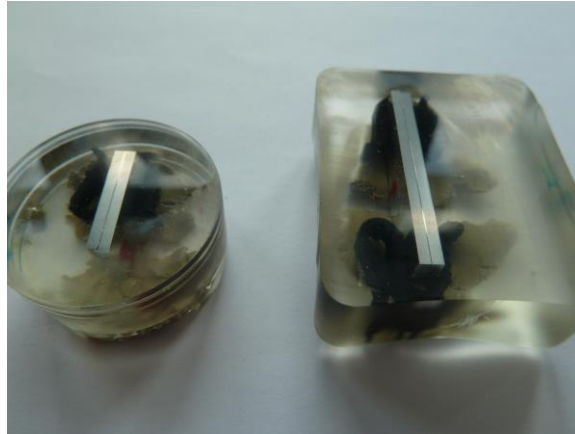
Figure 34 - Joined aluminium sheets moulded in epoxy.
