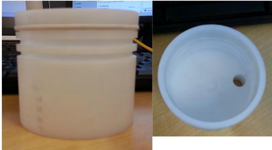
Figure 3.2.: The model of a piston made out of Delrin.
