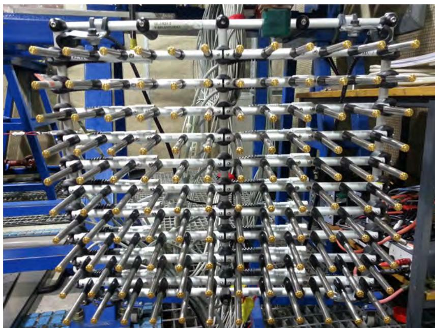
Figure 2.2.: The microphone array with 3 cm spacing.
