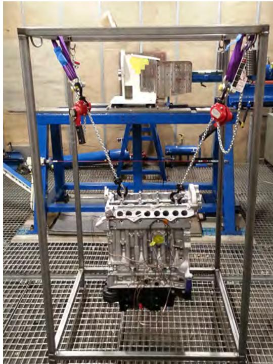
Figure 3.10.: The steel frame that the engine was hanged from during the measurements.
