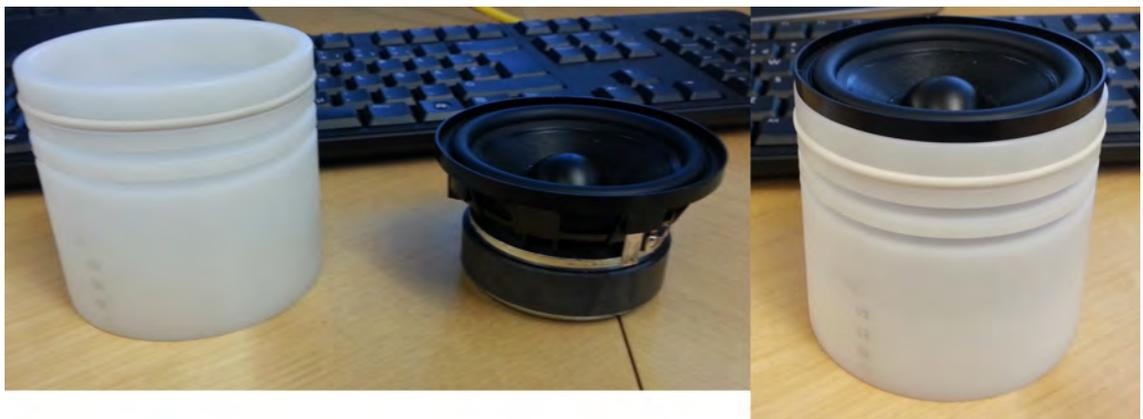
Figure 3.3.: The configuration with the loudspeaker element placed in the piston model.
