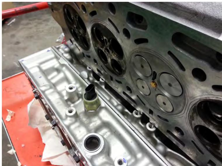
Figure 3.8.: The reference microphone placed at the injection nozzle position.
