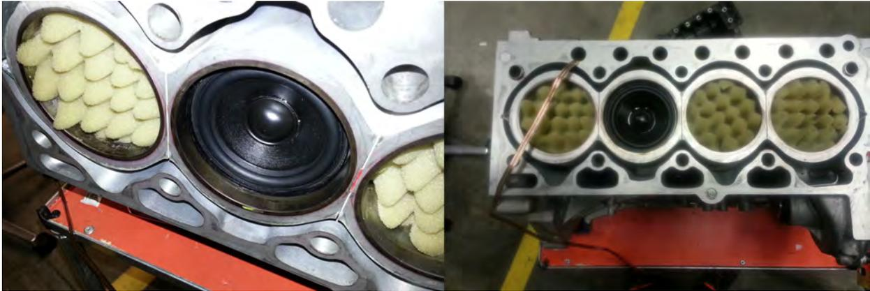
Figure 3.6.: The placement of the loudspeaker element inside the combustion chamber.
