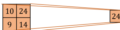
Figure 2.8: Figure of a 2x2 max-pooling with the input in the 2x2 grid to the left, and the output in a 1x1 square to the right.
