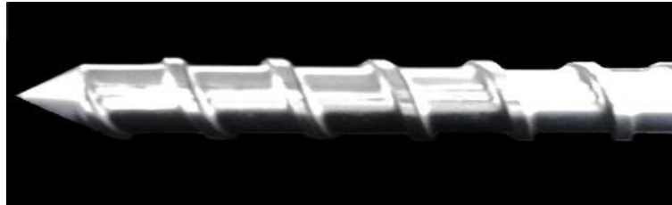
Figure 9. Detail of the ending part of the conventional screw used in this work.
