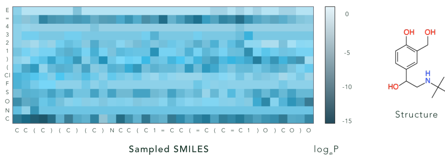
Figure 4.3: Generation of a new molecule. On the y-axis, we see the vocabulary and the conditional probability to sample each character at every generative step. On the x-axis, the sampled character at every step is shown. The graph of the generated molecules is displayed to the right.
