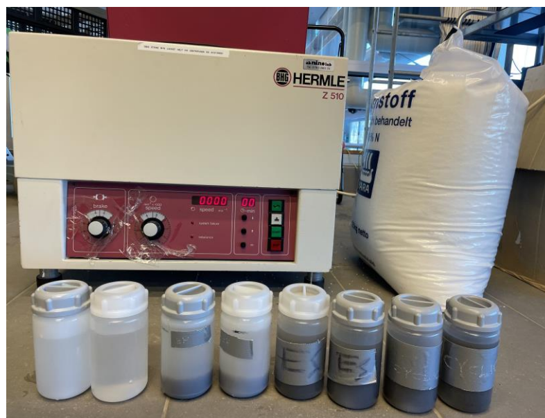
Figure 7. Centrifugator Hermle Z 510 and sludge samples after centrifugation.
