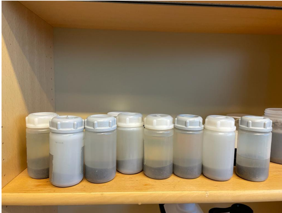
Figure 8. Mixed AGS-sludge samples after centrifugation.
