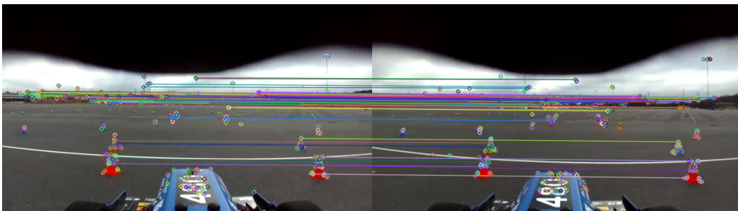
Figure 3.3: Keypoints found by ORB detector from OpenCV and filtered matches
