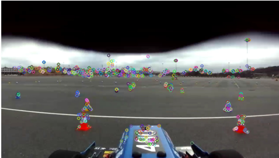
Figure 3.4: Keypoints found by ORB detector from OpenCV
