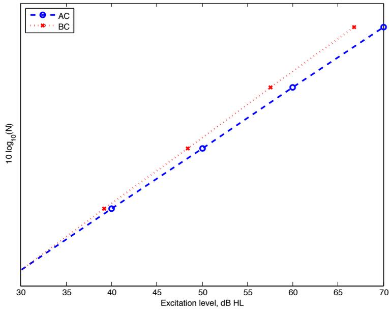
Figure 1.3.: The graphs show loudness functions for AC and for BC. The rightmost curve shows how the loudness function for AC, as described by Stevens power law and the exponent 0.30 (i.e.  $N \propto I^{0.30}$ ), looks like. By using the results in Figure 1.2, in combination with this loudness function for AC, the loudness function for BC is derived. The leftmost curve shows this function and its slope corresponds to an exponent of 0.33.
