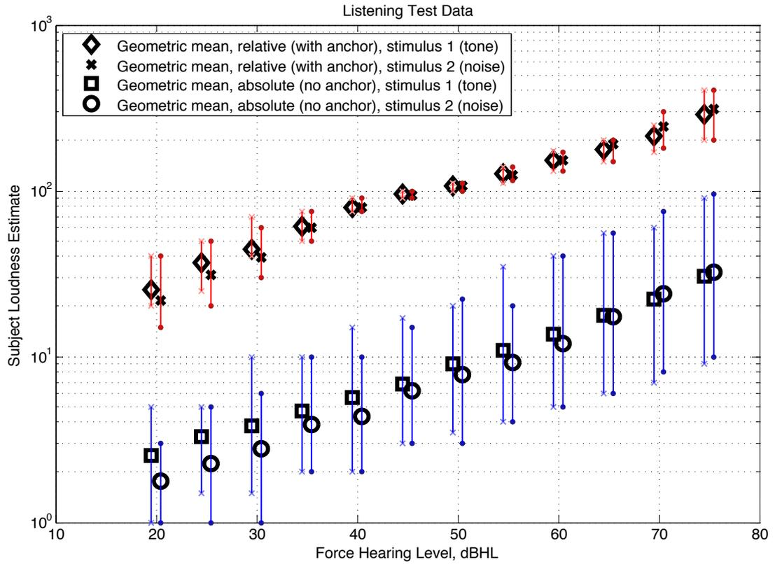
Figure 4.2.: Data from the listening test. The bold symbols (square, circle, diamond and cross) shows the geometric mean of the data. The vertical bars indicates inter quartile ranges. Stimulus 1 is a pure tone at 1 kHz and Stimulus 2 is noise with bandwidth 1 bark band around center frequency 1 kHz.
