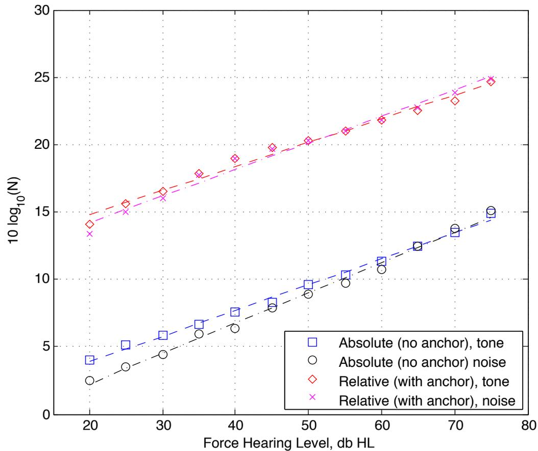
Figure 4.3.: Data from the listening test. The data point shows the geometric mean of the data and the dotted lines are curves fitted to these geometric means. The slope of the curves are:  $k = 0.19$  for Stimulus 1 without anchor,  $k = 0.23$  for Stimulus 2 without anchor,  $k = 0.18$  for Stimulus 1 with anchor and  $k = 0.20$  for Stimulus 2 with anchor.
