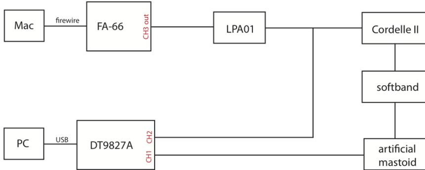
Figure A.1.: Setup during the measurement of  $F_{act}$  and  $U_{act}$ .
