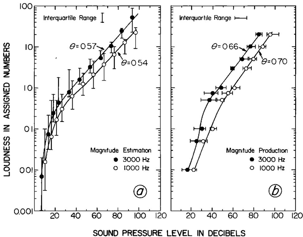
Figure 1.1.: The results from magnitude estimation and from magnitude production that was performed for AC[Hel 76]. The vertical and the horizontal bars show the interquartile ranges. The slope of about 0.6 is relative sound pressure. This corresponds to 0.3 relative sound intensity.
