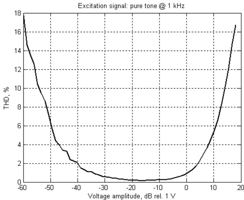
Figure 3.1.: Total harmonic distortion of the actuator as a function of the voltage to the actuator,  $U_{act}$ .
