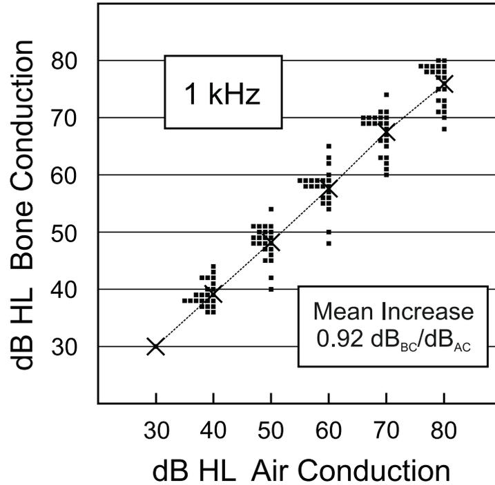
Figure 1.2.: Results that were obtained from the loudness balance test between AC and BC for the normal hearing group [StHå 01]. Individual results are represented by dots. The BC mean for each level is given by the crosses along the dotted lines.
