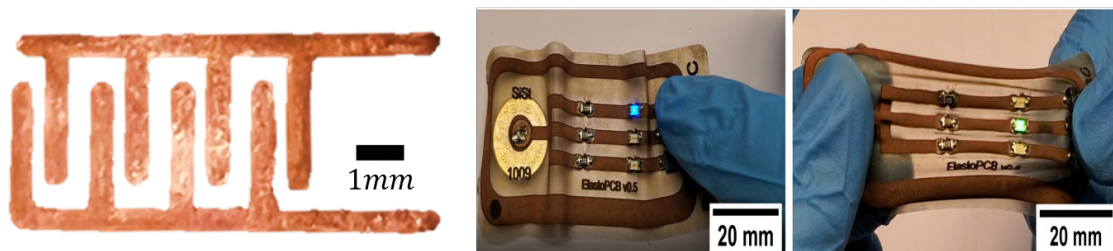
Figure 1.5: A pair of interdigitated electrodes made of pure Cu by ECAM (Left) and a stretchable circuit board made of Cu based material by ECD (Middle and right). (The image in the middle and on the right is reproduced from Ref.[24] with permission from MDPI)
