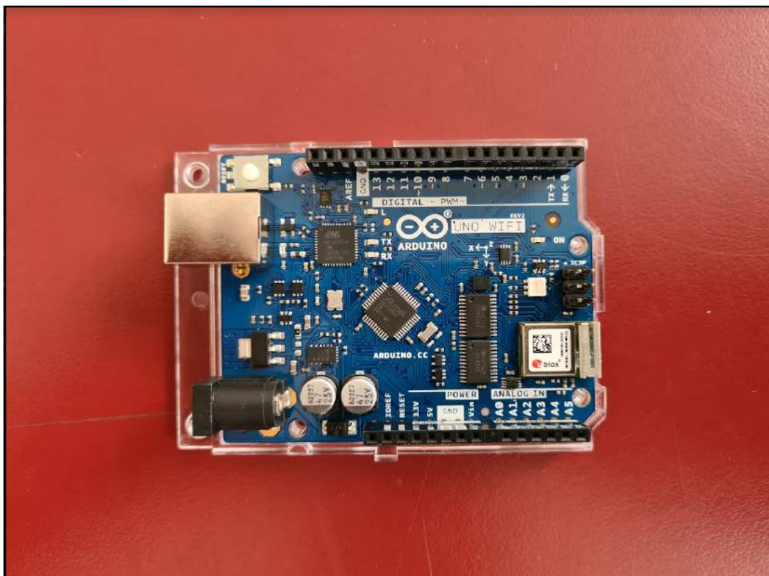
Figure 2.3: Arduino board to be used in the project
