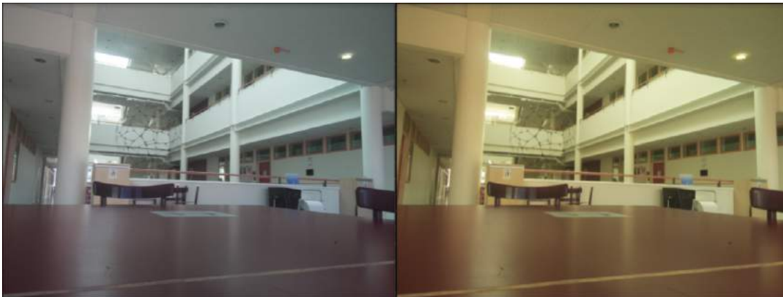
Figure 4.6: Before adjusting the AWB (Left) and After adjusting the AWB (Right)
