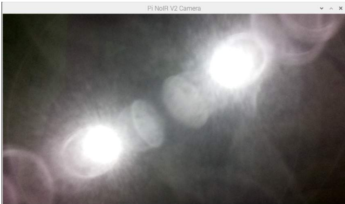
Figure 4.10: IR leds being illuminated directly on the NoIR camera
