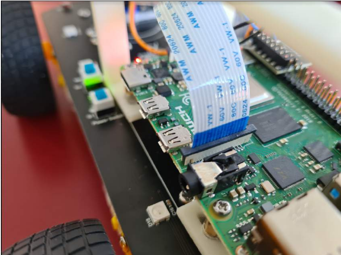
Figure 4.5: Connection of the Camera to the Raspberry Pi
