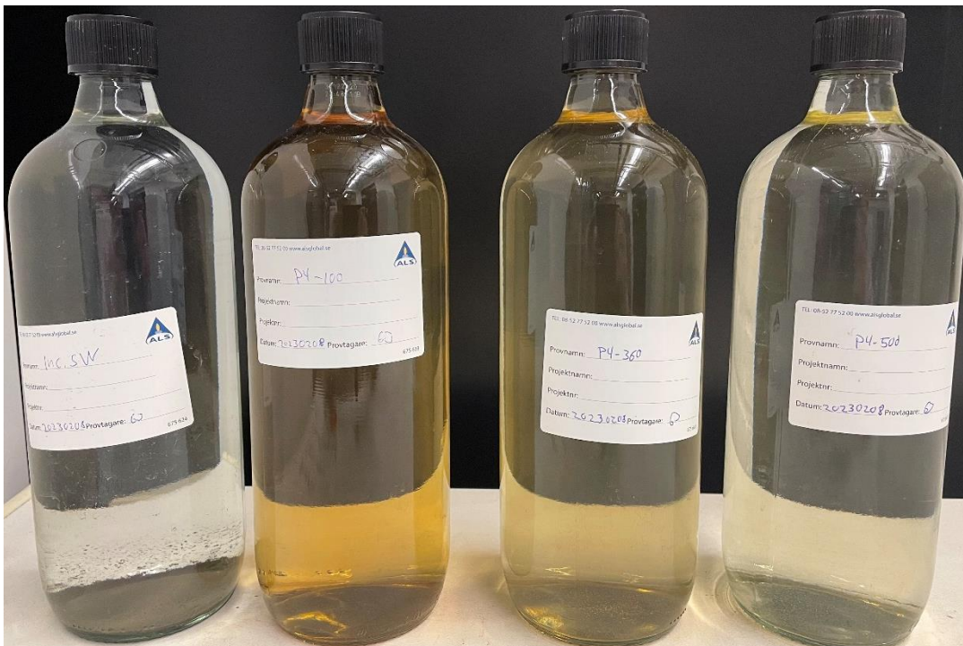
Figure 5. Samples from the peat filter after addition of 100L, 360L and 500L of polluted stormwater compared with incoming stormwater in the bottle to the left.
