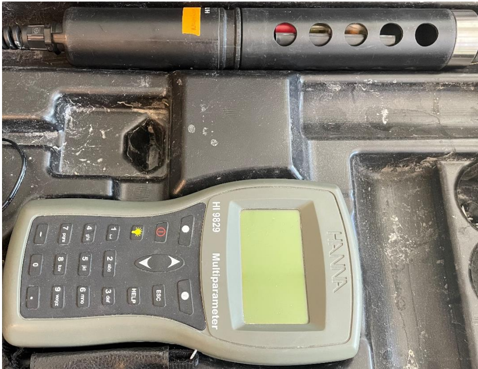
Figure 4. The Hanna multimeter instrument (HI 9829) used for the measurement of pH, redox potential, conductivity and turbidity.
