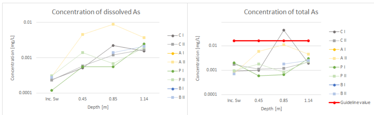
Figure 9ab. The concentrations of dissolved and total As variation by depth in the filters and sampled passively.
