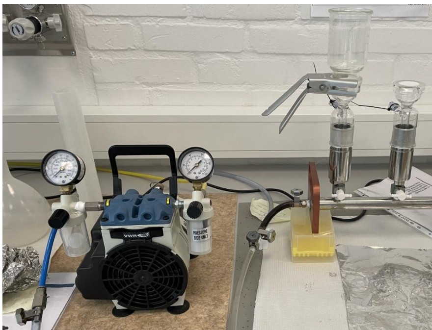
Figure 6. The setup used for filtration when measuring TSS and VSS.
