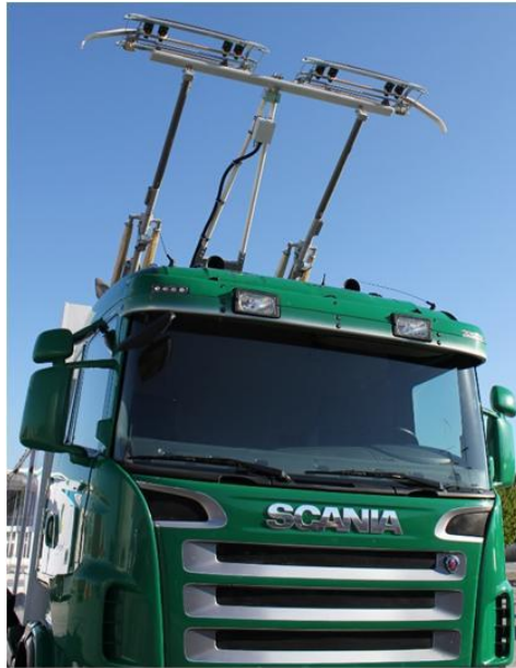
Figure 3-7 Conductive power transfer from overhead catenaries (Scania)
