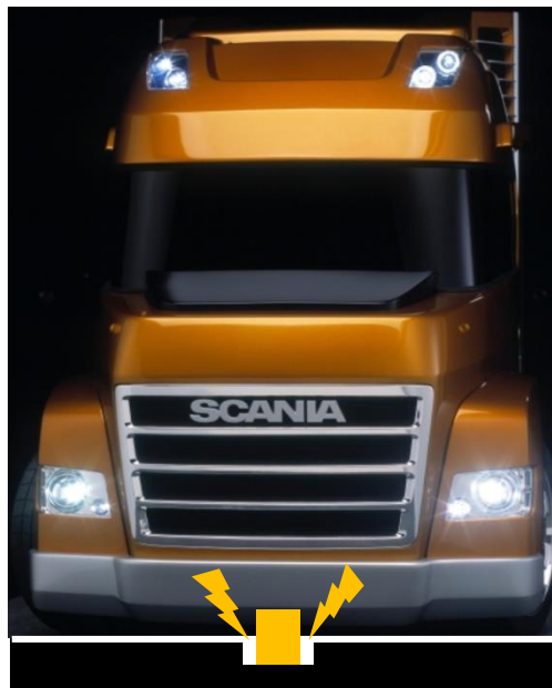
Figure 3-8 Conductive power transfer from the road (Scania)
