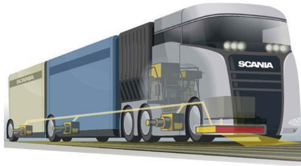
Figure 3-9 Inductive power transfer from the road (Scania)
