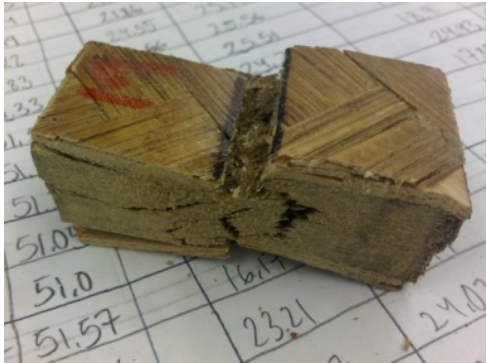
Figure 4.14 Failure in shear perpendicular-to-the-plane
