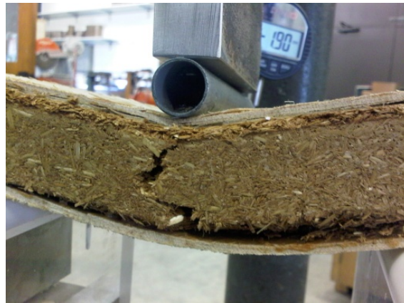
Figure 4.1 failure in bending test
