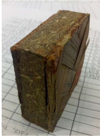
Figure 4.9 Failure compression parallel-to-the-plane
