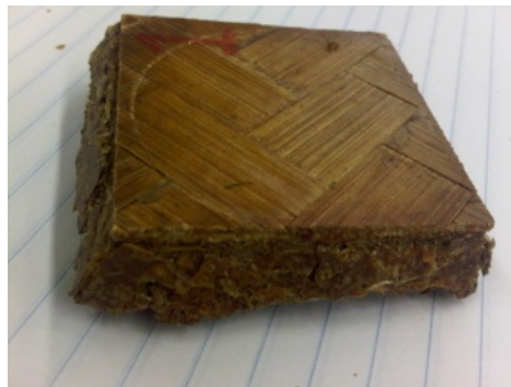
Figure 4.7 specimen after testing in compression perpendicular-to-the-plane
