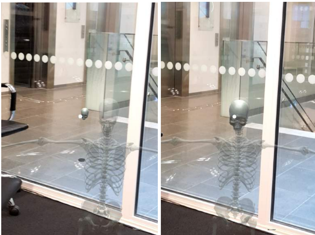
Figure 6.25: The solution in LumbAR for the problem with depth perception, where the piece the user holds snaps to the same depth as the skeleton when looking at it.
