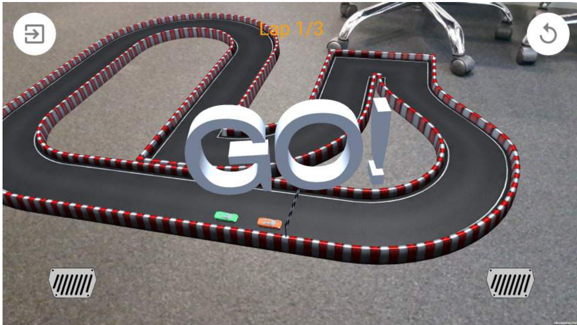
Figure 6.23: The countdown in AR-Racing is always facing the user, and the rotation is therefore not synced between the different devices.
