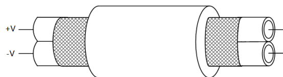
Figure 3.5: twinaxial cable short-circuit
