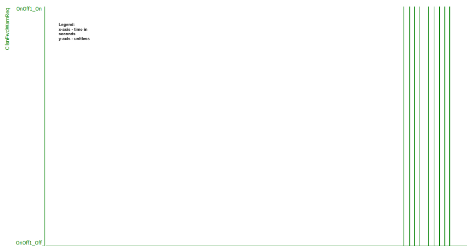
Figure 4.8: This graph indicates a Collision forward warning request signal that gets activated when an object is placed in front of it. It goes high for an object in front of it and goes low when it disappears.
