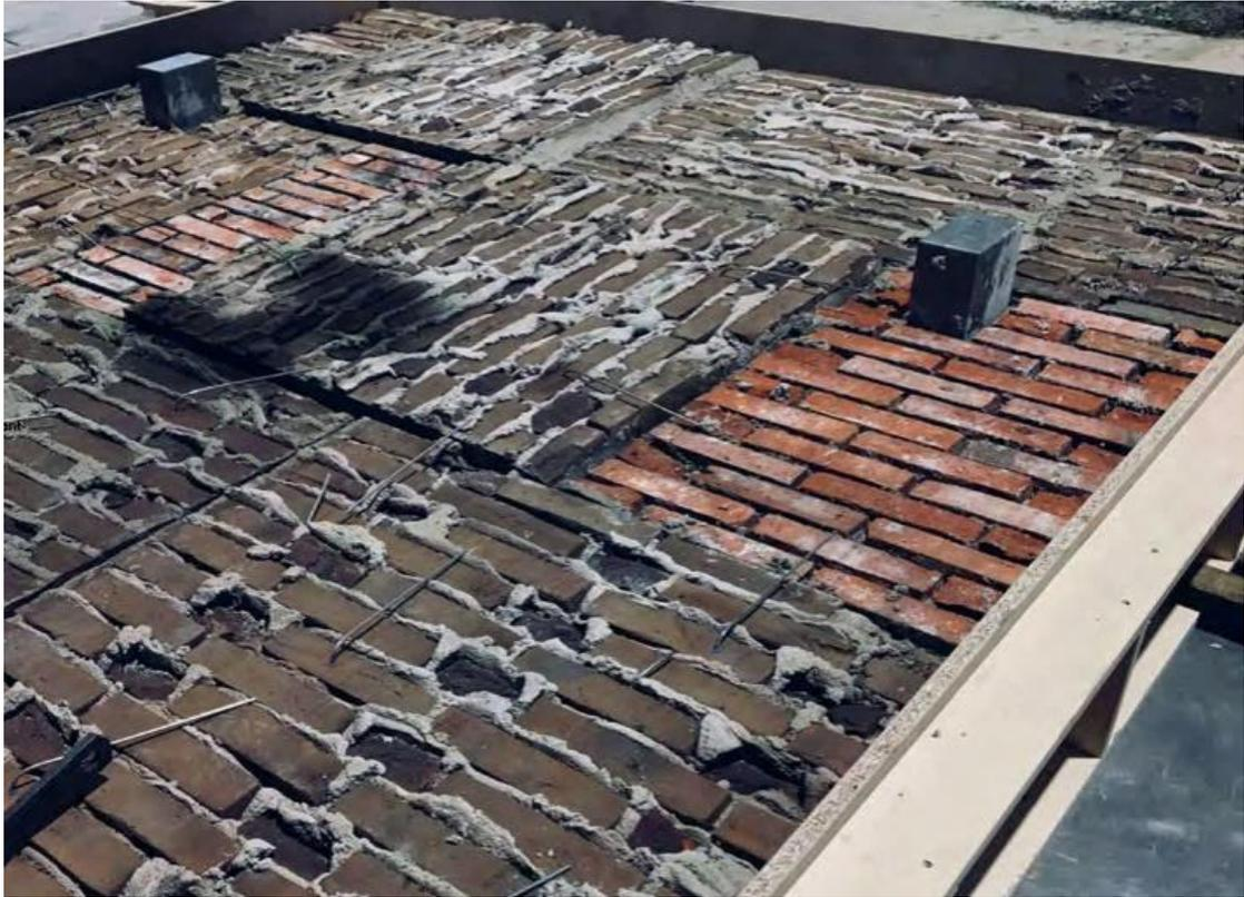
Figure 2.9 Brick modules in a mould on which concrete was cast. Reprinted with permission from Lendager Group.
