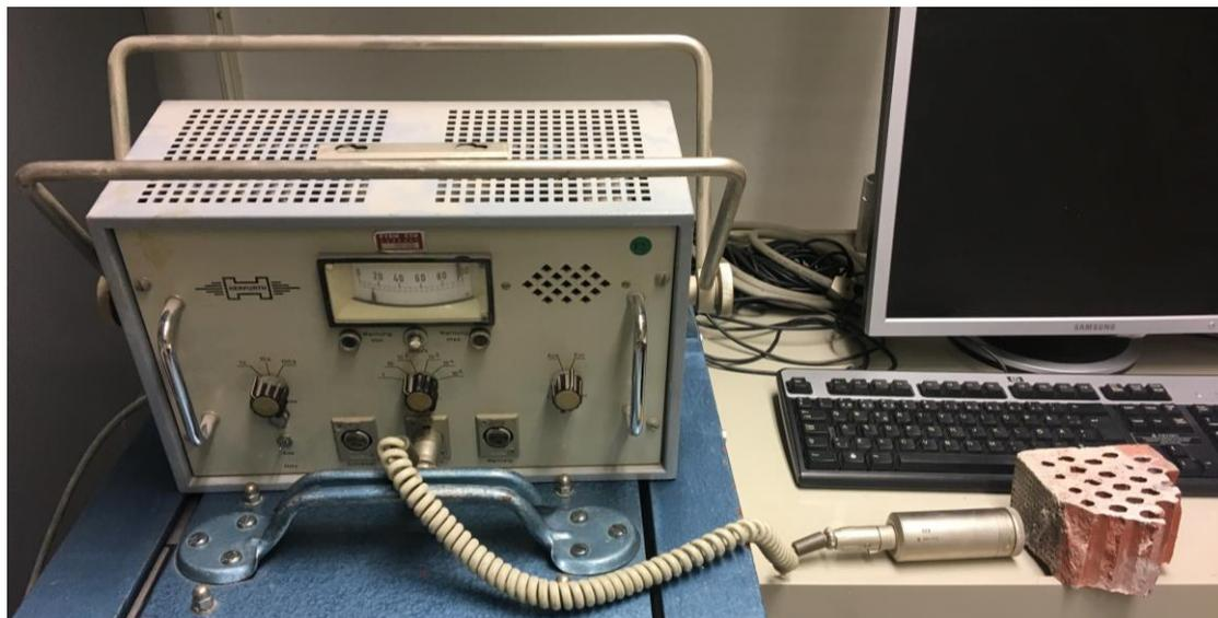
*Figure 3.5* Radioactivity test setup. The Geiger counter to the left and the brick sample to the right. The test showed that the brick is not radioactive.
