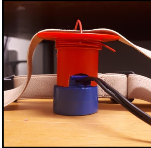
Figure 3.3. Plastic extension with a small opening for wires.
