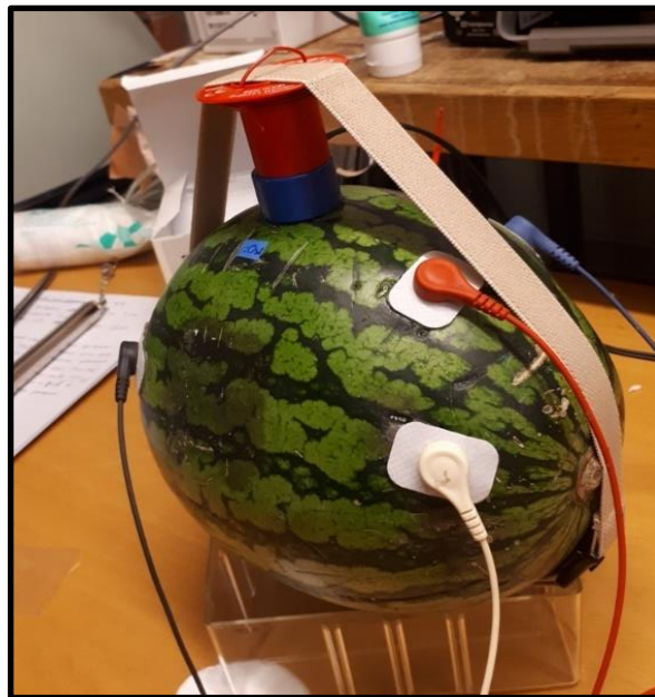
Figure 3.6. Electrode placement in synthetic cVEMP, S1. The artificial head is in horizontal position. Red bipolar electrode placed on the artificial SCM muscle, ground electrode on the virtual forehead.
