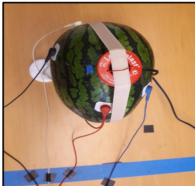
Figure 3.8. Electrode placement synthetic ABR, S1. Artificial head in horizontal position (From above). Red bipolar electrode on the synthetic mastoid. White bipolar electrode is placed approximately 3.5 centimeters from the ground electrode.
