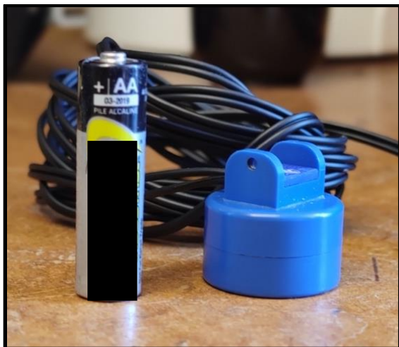
Figure 2.5. (Left) AA+ battery for size comparison and (Right) the transducer B250 prototype. A steel spring arrangement is attached using the small cavities on the top of the B250.
