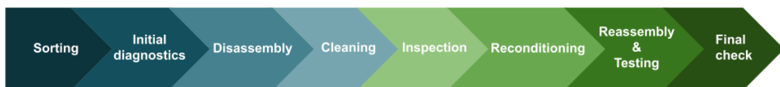
Figure 2.4: The remanufacturing process and its general steps within automotive industry (adapted from ERN, 2016a).
