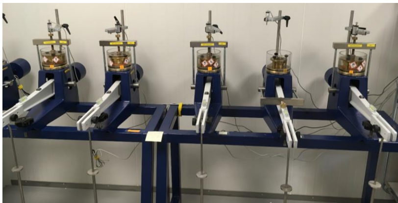
Figure 33. Setup of oedometer testing for determine the increase in stiffness.
