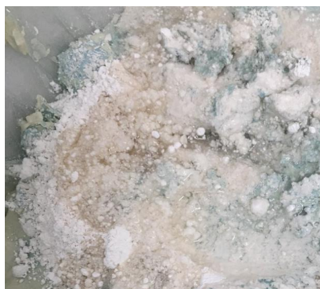
Figure 30. Reaction of Ca(OH)_2 and SiO_2 , making the slurry brown at some locations with high concentration Ca(OH)_2 .
