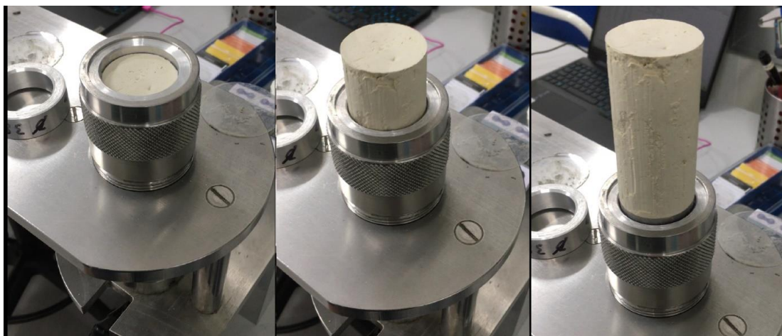
Figure 25. Extraction process of a sample, note the metal disk pushing out the sample in the picture to the right.
