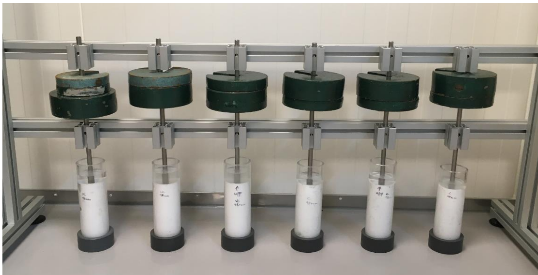
Figure 27. Samples prepared by having a weight of 6 kg, corresponding to 50 kPa at an estimate soil depth of 3-4 meters. Note that the samples were not wrapped in plastic.
