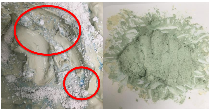
Figure 28. Start of mixing with calcium hydroxide (left), finished mixing after 10 minutes (right). Note the how the colour differs at the locations where the clay is in contact with the calcium hydroxide (marked in red), indicating production of copper hydroxide.
