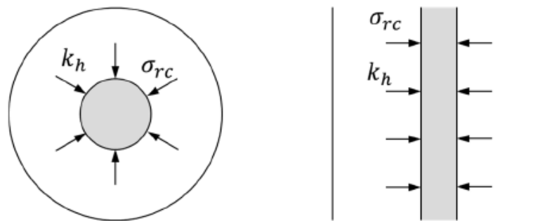
Figure 23: Column confining and seepage pattern vs trench confining pattern (adapted from Castr,2017)
