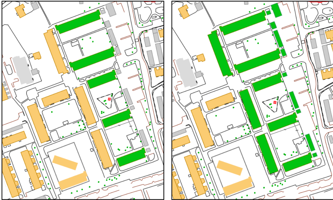
Figure 4.6: Buildings with green roofs. The figure to the left corresponds to the 5th percentile flow and the selection of buildings given green roofs is a proposal. The figure to the right shows that all buildings in the catchment area are given green roofs which corresponds to a flow of 179 l/s which is the 15th percentile flow retrieved from @Risk.
