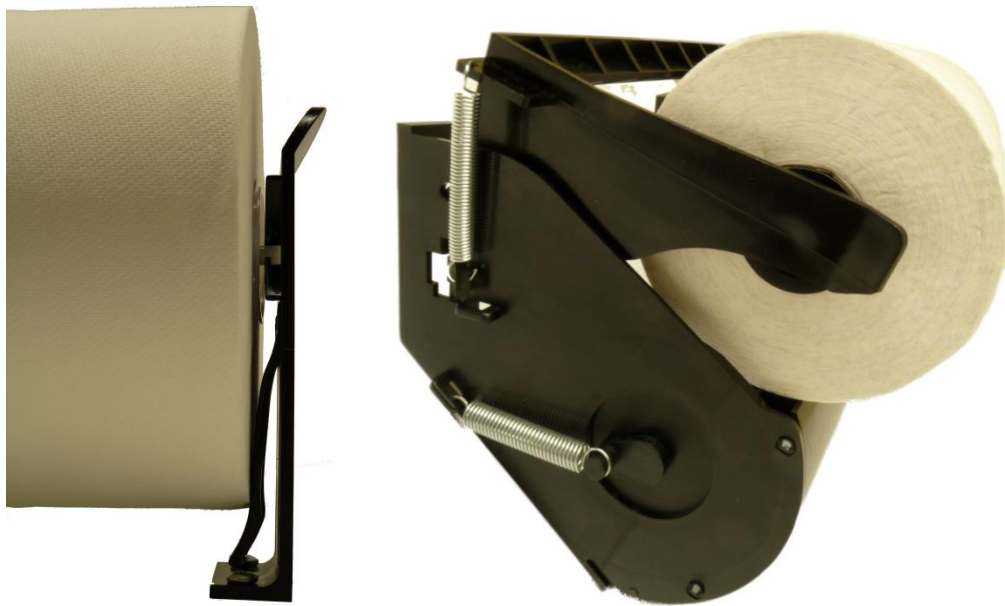
Figure 20: Brake mechanisms, Left: brake block, Right: roll direct onto cutting cylinder.
