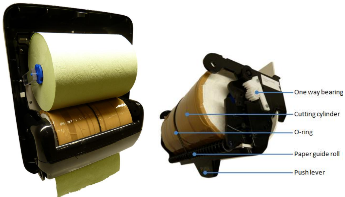
Figure 28: Physical appearance model, the brown taped paper roll visualizes the cutting cylinder
