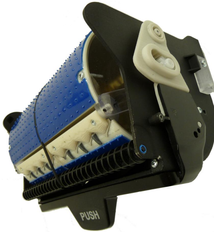
Figure 43: Prototype without front covers, the emergency push lever with the cogwheel and the knife are visible.
