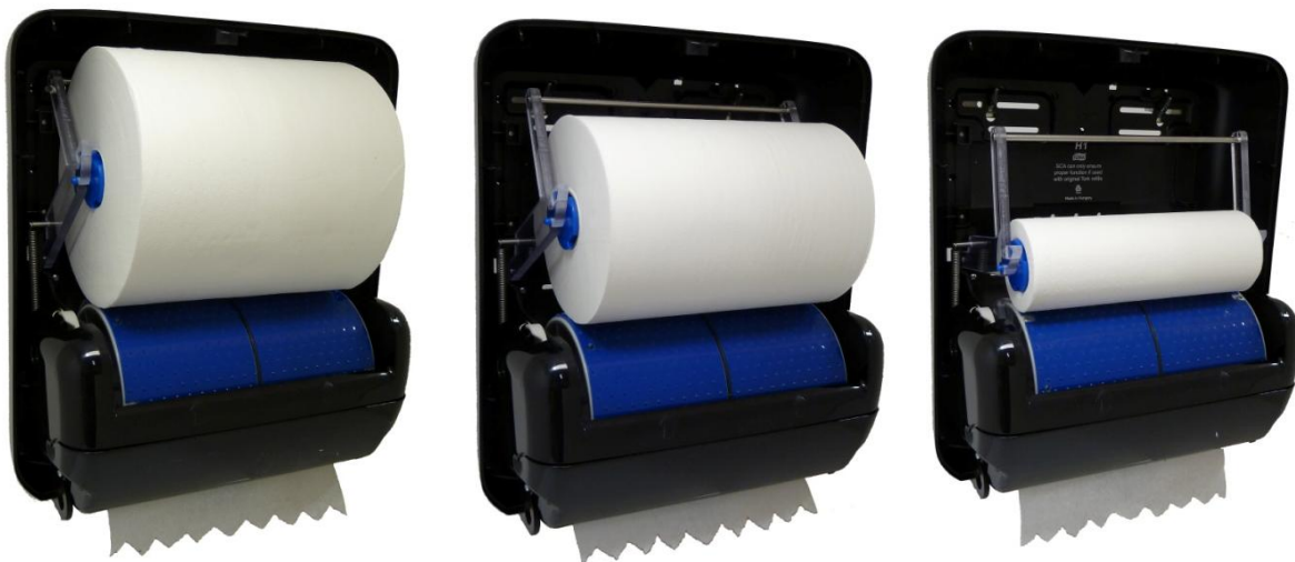
Figure 44: Testing of prototype, Left: Full roll, Middle: Half full roll, Right: Nearly empty roll.
