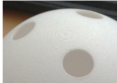
Figure 46. Detail of hole in the Prototype 1 Figure 47. Detail of layers visible on Prototype 1 surface
