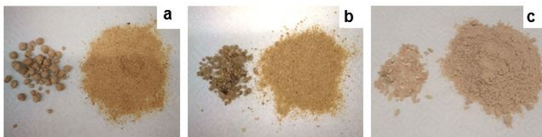
Figure 5.1: a) DRB (defatted rice bran), (b) HSRB (heat stabilized rice bran) and (c) UPRB (unprocessed rice bran). All are divided into fractions above d=2\text{mm} (left) and below d=2\text{mm} (right).
