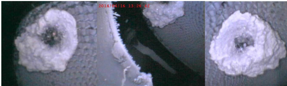
Figure 4.23 Deposits on substrate on high point with 6-hole injector
