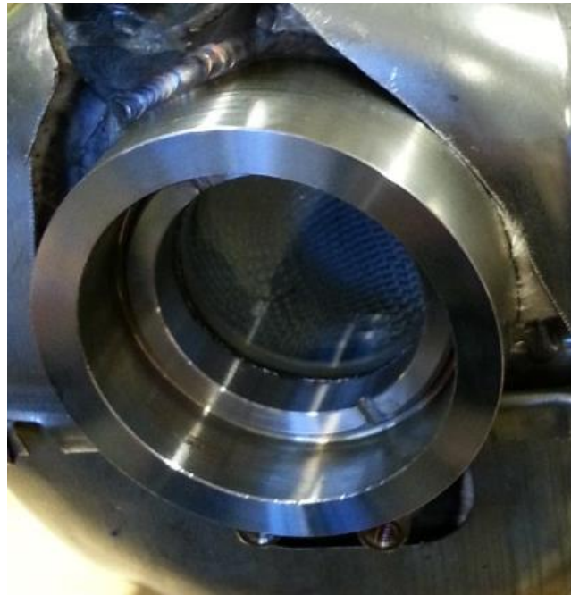
Figure 3.2 Inspection glass on the substrate side
