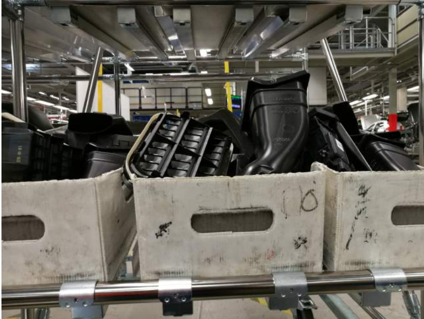
Figure 3.14: Kitting boxes that are filled with components and stored in flow racks.
