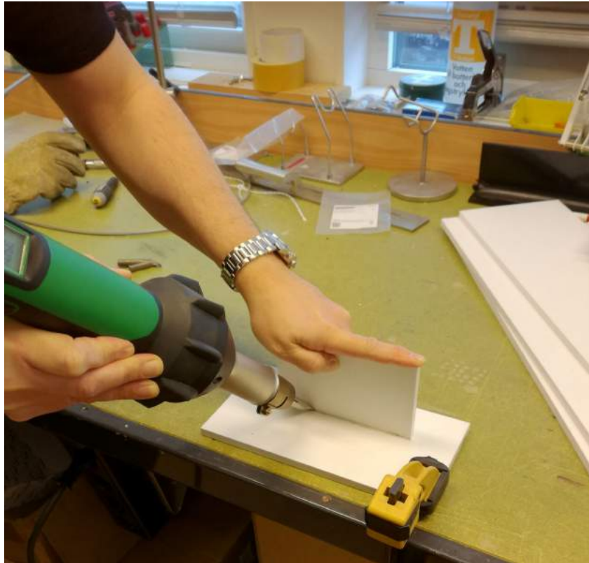
Figure 7.10: The process of pre-jointing the materials.
