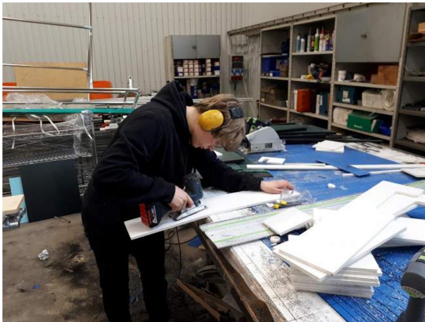
Figure 8.1: A jigsaw was used to create handles and other contours.
