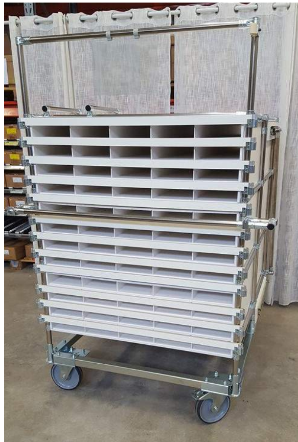
Figure 1.3: A kitting trolley with a shelving system that is made in PVC-foam.
