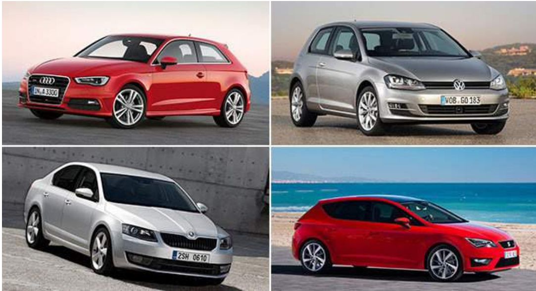
Figure 3.4: Four cars from different brands that have the same platform. [24].
