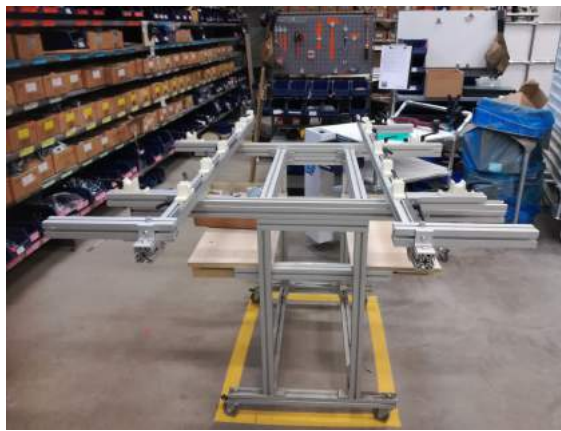
(c) An auxiliary tool is used to assemble the steel frame.
