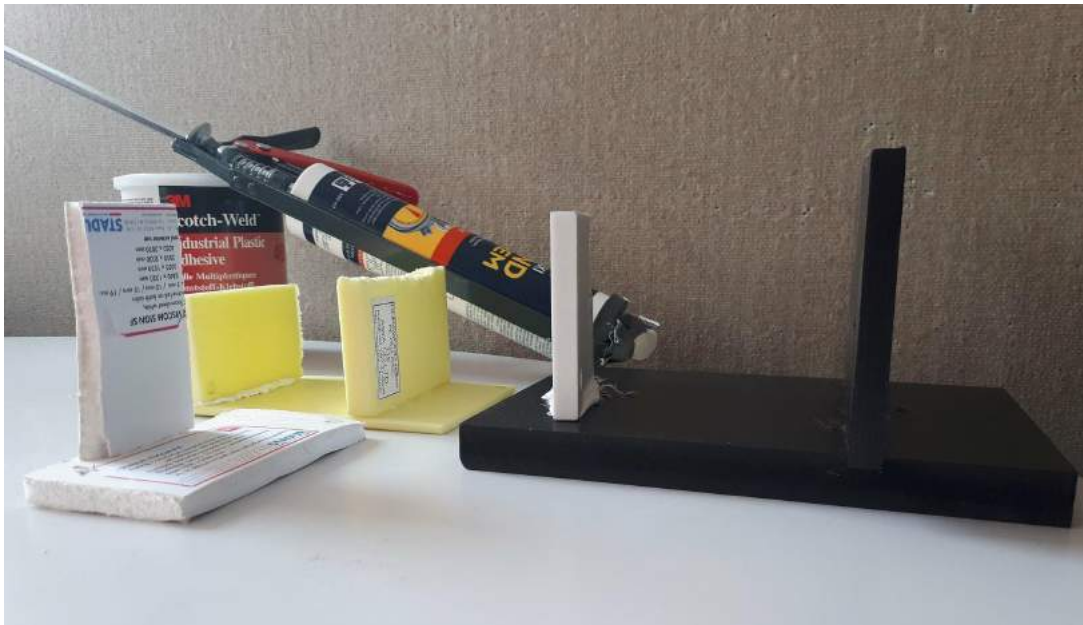
Figure 7.14: Part of the testing of three different glues together with three different plastic materials.
