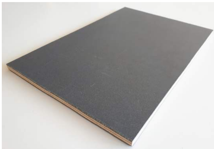
Figure 9.8: The plywood covered with PP with a total thickness of 9 mm.
