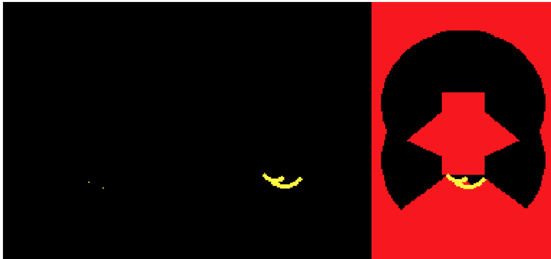
Figure 3.6: USS data occupancy representations to be used as training data, where yellow denotes occupied cells, black is free space and red is unknown. Left: sparse basic, middle: sparse arc, right: dense arc.
