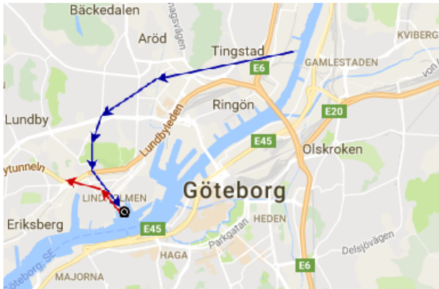
Figure 4.7: Example of a machine learning algorithm predicting a user’s trajectory. User is denoted by black circle, previous movements by blue arrows and predicted movements by red arrows. Here, t_{before} = 5 and t_{after} = 2 , background courtesy of Google Maps.
