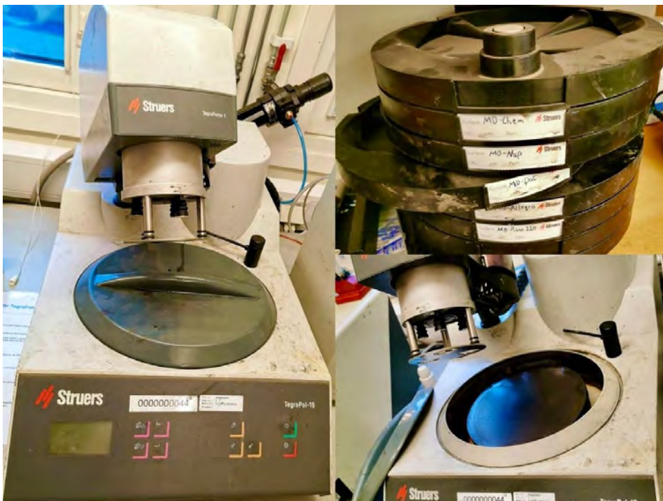
Figure 11- Struers TegraPol-15 machine (lid closed to keep the machine clean) along with polishing blade container and the polishing machine with open lid.
