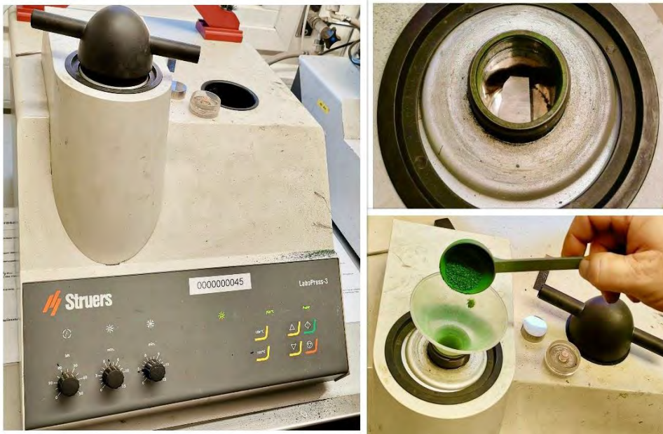
Figure 10- Struers Labopress 3 casting machine along with sample placing and addition of the plastic powder
