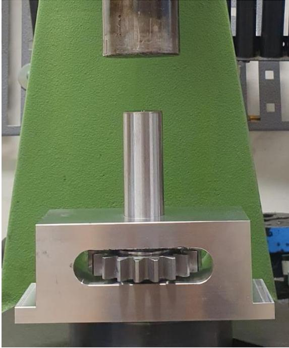
**Figure 23:** Before shaft press fit.
