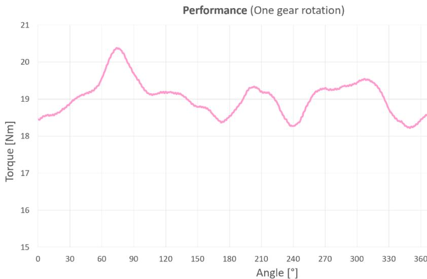
**Figure 37:** Plot of one full gear rotation.
