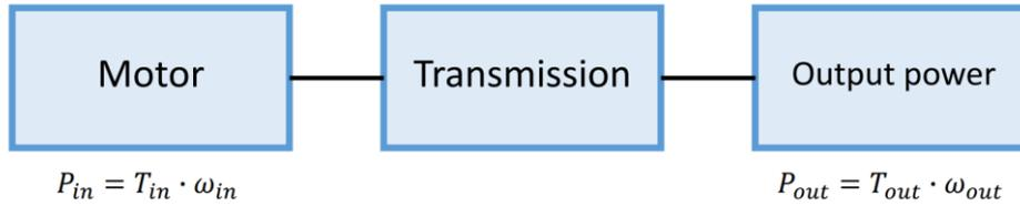
**Figure 4:** Theoretical illustration of the mechanical transmission in the GFA.
