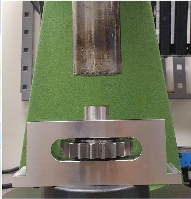
**Figure 24:** After shaft press fit.
