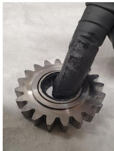
**Figure 22:** Lubrication after press fit.
