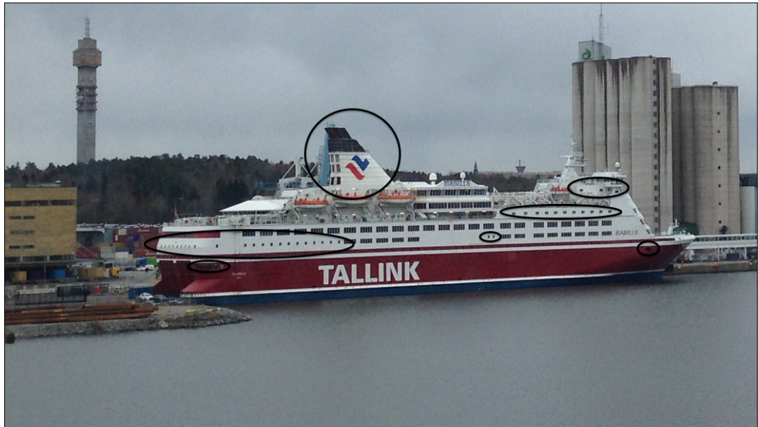
Figure 3.1.: The main contributors of the direct airborne noise are marked with black.
