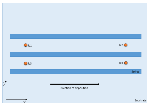
Fig. 3.2 yx -view of geometrical dimensions and placements of the thermocouples T_{c1} , T_{c2} , T_{c3} and T_{c4} of process trial E_2 .
