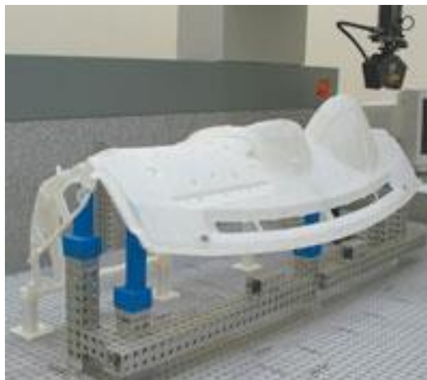
Figure 5 - FDM Dashboard Prototype Holds Tight Tolerances; Improves Design (Stratasys, 2017).
