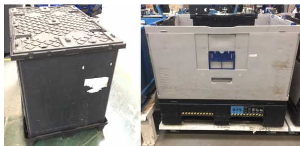
Figure 5.20. One stackable plastic pallet with lid and walls (left) and one with a flap on side for easy picking (right).
