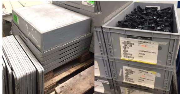
Figure 5.23. Empty nestable containers (left) and stackable plastic containers with plastic parts (right).
