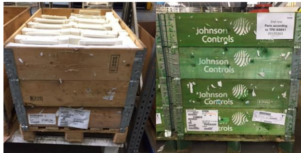
Figure 5.19. Low-collar wooden pallet (left) and high-collar wooden pallet (right).
