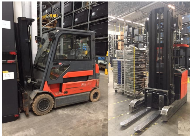
Figure 5.16. Counterbalanced forklift (left) and reach forklift (right).
