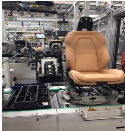
Figure 5.3. Kitting box on the assembly line next to a front seat.
