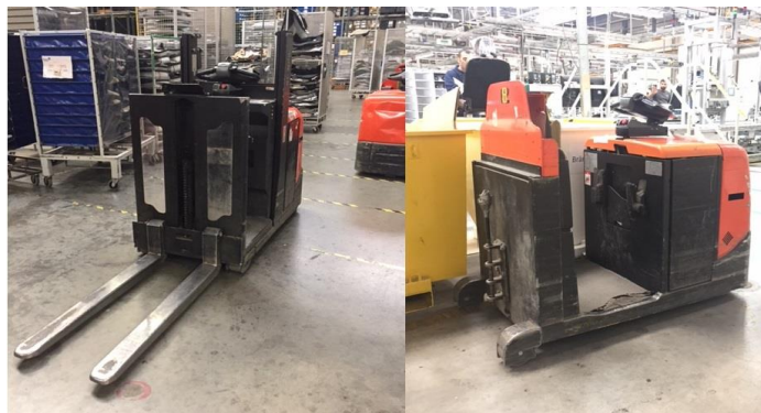
Figure 5.18. Platform powered pallet forklift (left) and electric tow tractor (right).
