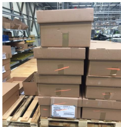
Figure 5.22. Unwrapped wooden pallet unit load of cardboard containers with detachable lids.
