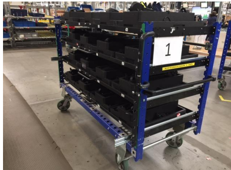
Figure 5.2. One of four wagons on which kitting boxes are placed for delivery to assembly.
