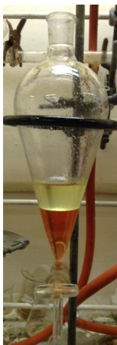
Figure 49. The first shaking of styrene with sodium hydroxide to remove its inhibitor (4-tert-butylcatechol )
