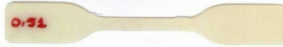
Figure 45. A standardized tensile test specimen of a copolymer of benzyl starch with 50 % (w/w) HIPS
