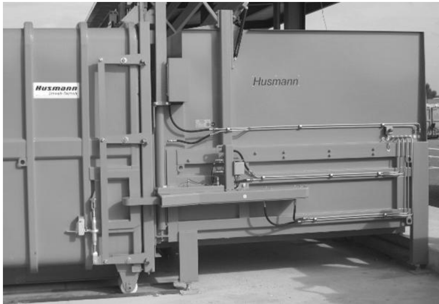
Figure 21: Example of stationary compactor with attached container.
