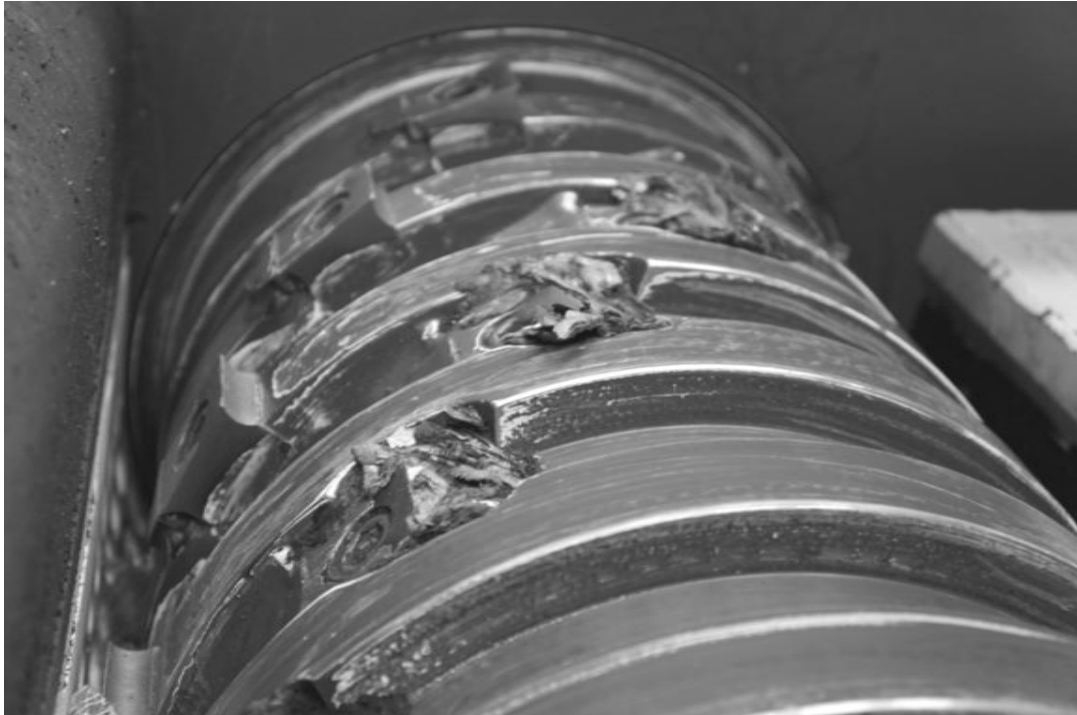
Figure 17: Picture of material stuck on the knives on supplier 1's shredder.
