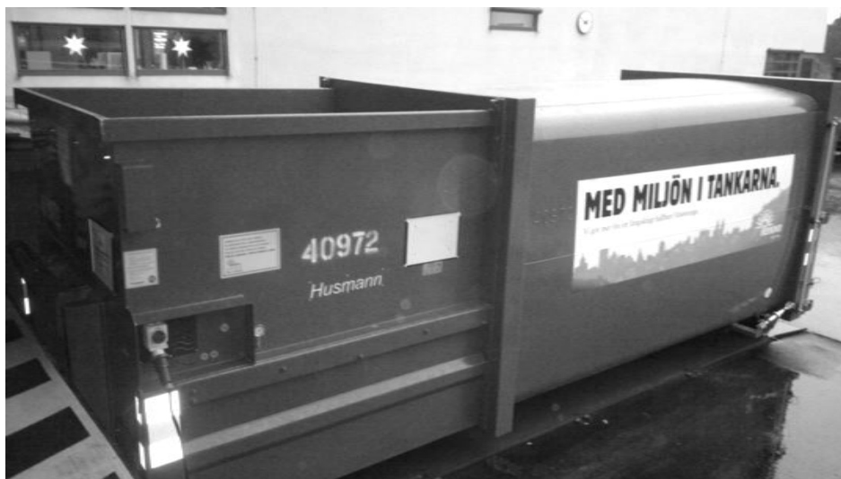
Figure 3: Compactor for corrugated cardboard and burnable waste.
