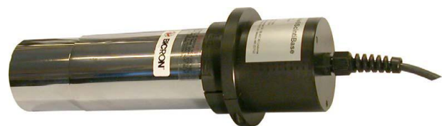
Fig 11: Scintillator connected to the Scintibase
