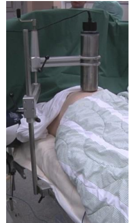
Fig 13: Scintillator connected to the patient during surgery above the heart
