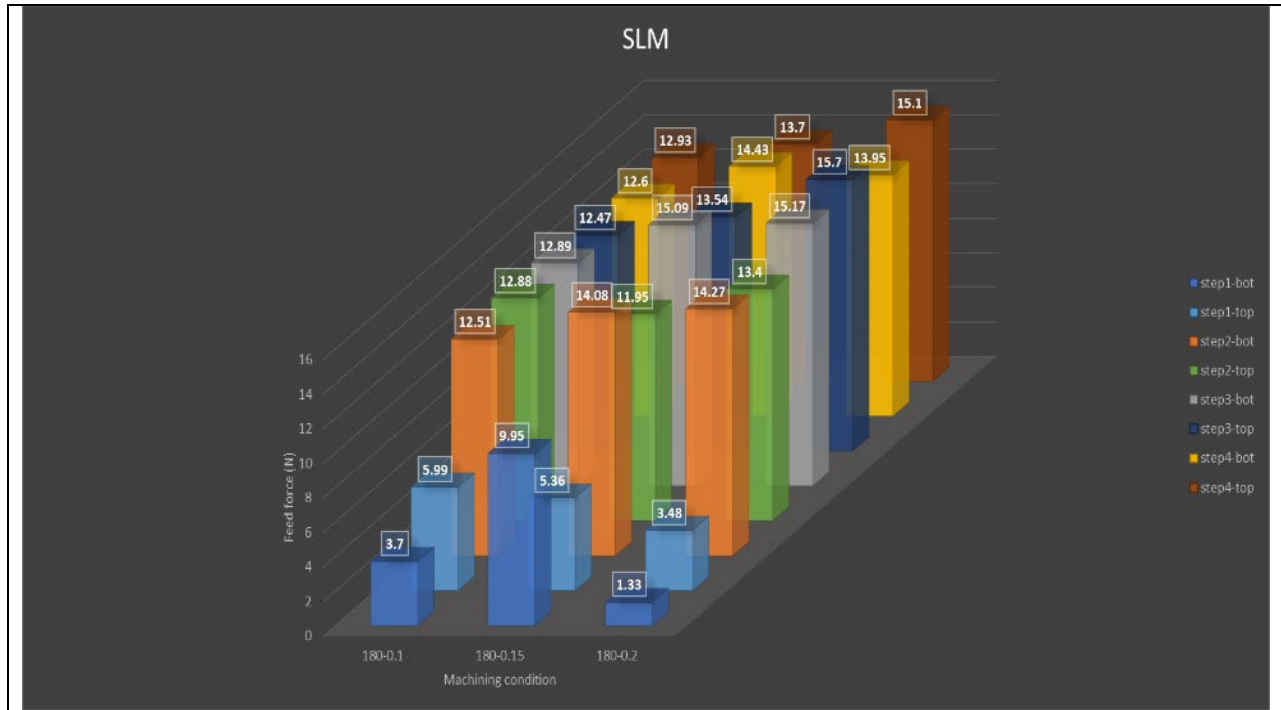
Figure 51: Feed force values for SLM part including 4 steps and different machining conditions.
