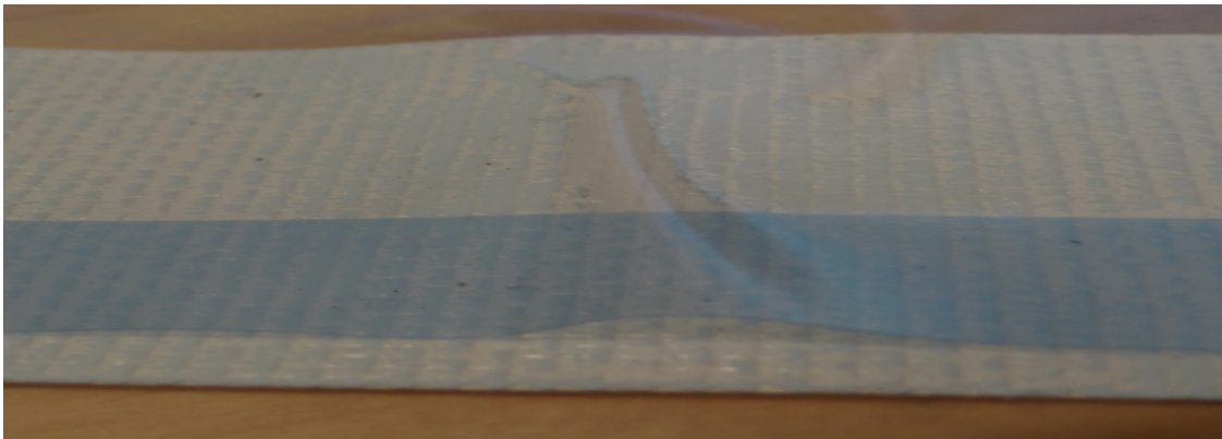
Figure 34. An illustration on how initiated channelling between tape and construction film looks like. Keep in mind that the materials in the picture were not included in this study. The initiated channel formation is a set up for demonstrational purpose.
