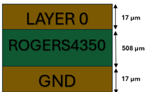
Figure 3.2: Three-layer PCB stackup with Rogers 4350 dielectric and copper layers.
