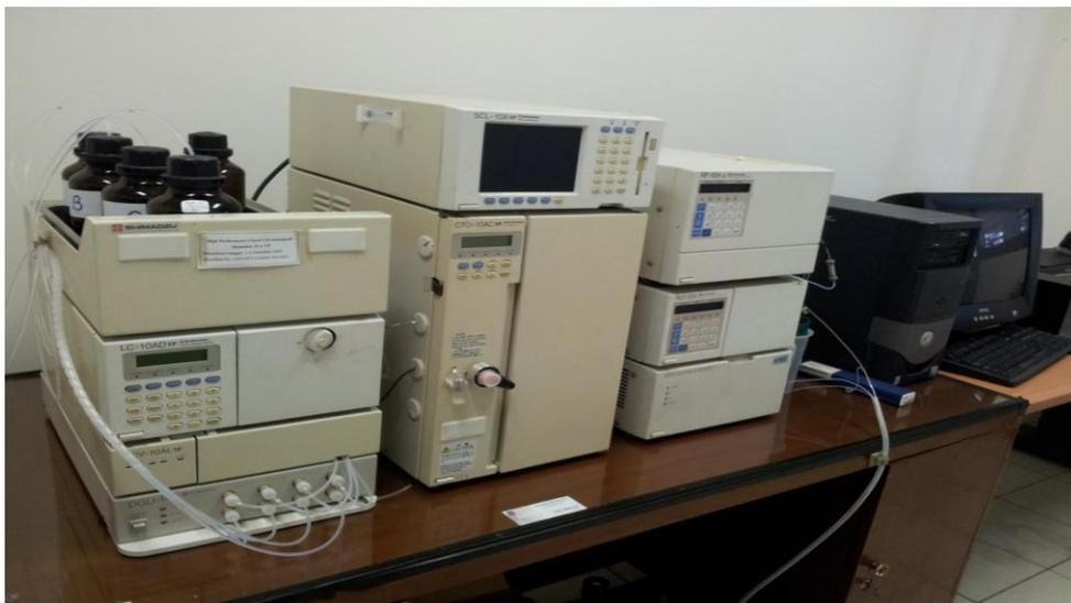
Figure 11: Showing High Performance Liquid Chromatography instrument with PC
