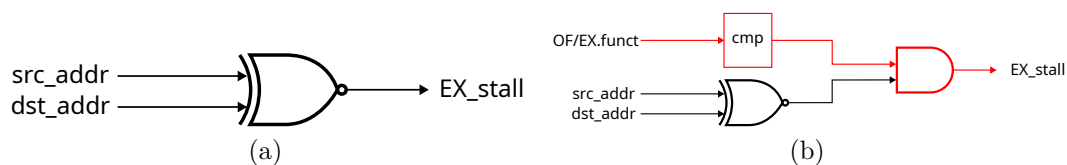
Figure 4.16: Data hazard detection in the RVV pipeline. (a) without EX forwarding and (b) with EX forwarding. The red sections indicate the additional hardware necessary for EX forwarding.
