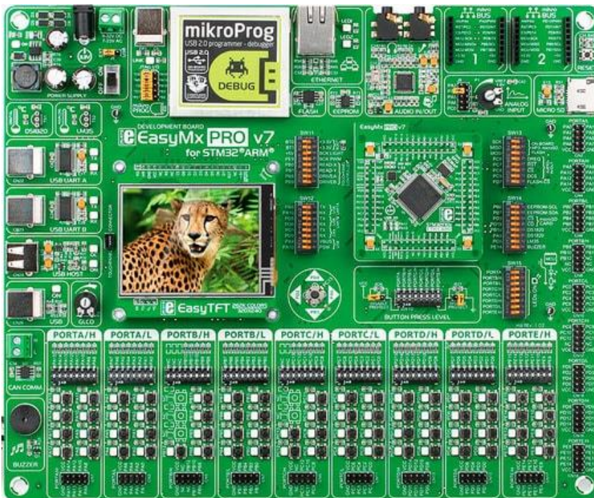
Figure 8 Easy MX PRO v7 Development Board
