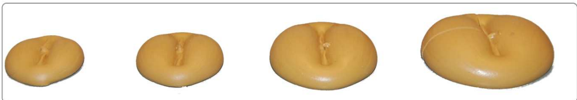
Figure 4-16: Real beads created by static and flat stream applicator
