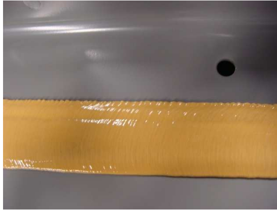
Figure 4-14: The outer surface of the selected beads
