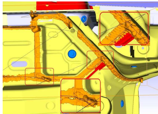
a: sealing beads underneath the car in simulation
