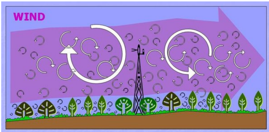
Figure 6 Eddy covariance measurement schematics. Tower for various altitude gas concentration measurements and eddies above canopy.
