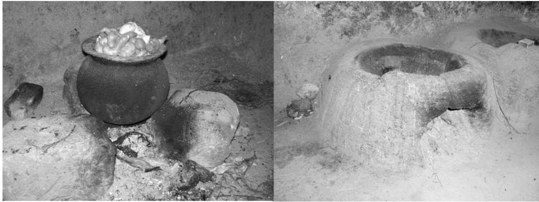
Figure 17. A traditional Kinyarwanda stove, which consists of three stones to the left. A fuel economic rondereza, which has circular walls to the right.
