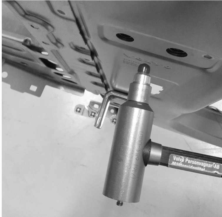
Figure 3.9. Impact hammer with a tip, load cell and mass.
